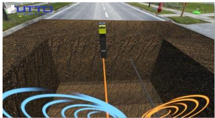
UTTO's VR simulation modes create locate experiences as if the field technician is in the real world. The locate device integrates with the virtual transmitter and behaves as if it were detecting pipes and cables under true electromagnetic signal conditions (both simple and complex).
